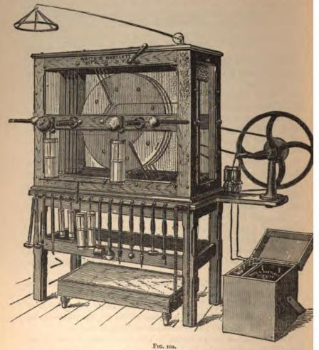
Holtz Static Induction Machine (with six 26-inch revolving plates, and sets of Electrodes and Leyden jars, with attachments for giving the static induced current, and insulated platform. The machine may be run by electricity from the street, by water, by hand, or as shown in the cut by a storage battery). For a description of the storage battery see Chapter II., Electro-surgery.
